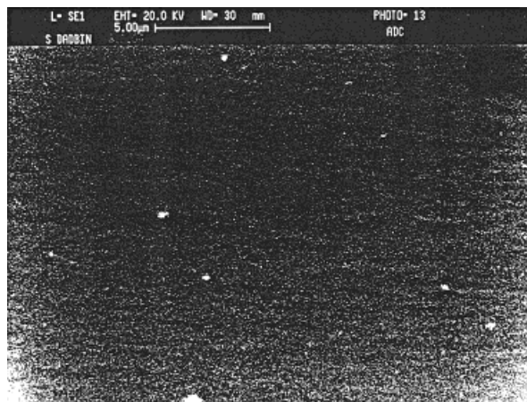
Figure 15 The SEM fracture surface of the ADC network (original magnification \times 5000 ).
